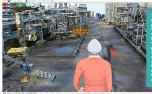
The 3D visualization of a brownfield plant made possible by COMOS Walkinside is used not only for planning and monitoring. Rather, it can also be used for training and operating purposes. For example, maintenance and repair tasks can be planned, simulated, and executed efficiently. The basis for this is the 3D engineering data from the basic and detailed engineering phases
